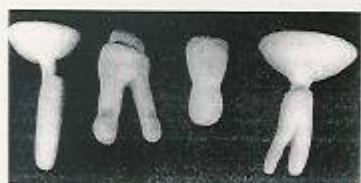
Fig. 30. Crude dental root implants made of machinable, highly bioactive glass ceramic. The implants were prepared by a centrifugation technique (Doz. Dr. R. Pinkert, Medizinische Akademie Dresden).
