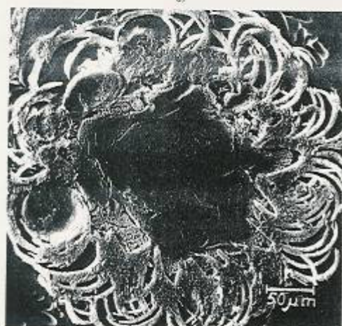
Fig. 6. a) Cordierite crystal as a defect in a technical glass (optical photomicrograph). b) Cordierite crystal in the new machinable glass ceramic that still has curved phlogopite mica crystals (scanning electron micrograph).
