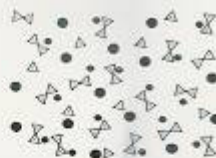
Fig. 17. Hypothetical model for the structure of a phosphate invert glass. Triangles, [\text{PO}_4] tetrahedra; black circles, cations ( \text{Na}^+ , \text{Ca}^{2+} , \text{Al}^{3+} ).
