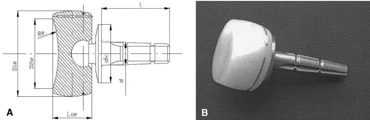
**Figure 6** The new prosthesis: Assembly drawing (A) and general view of the implant (B).  $D1e$ , diameter of the head;  $D2e$ , diameter of the articulate surface;  $Re$ , radius of the articulate surface;  $Loe$ , height of the head;  $dk$ , diameter of the collar;  $d$ , diameter of the stem;  $l$ , length of the stem.
