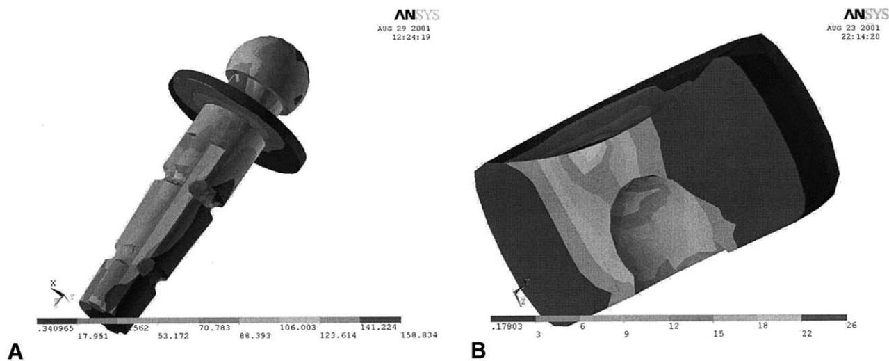
**Figure 4** von Mises stress plot in the prosthetic stem (**A**) and head (**B**) for a load of 687.75 N.
