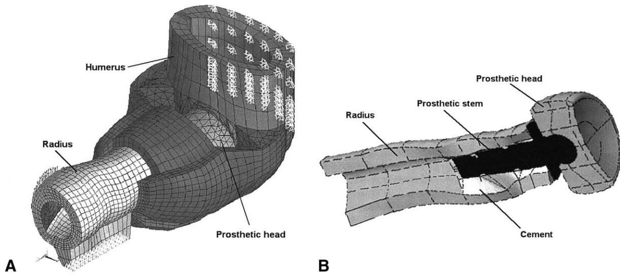
**Figure 3** Finite element model: Part of the elbow with prosthesis (**A**) and prosthesis fixed in the radius (**B**).
